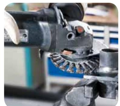
Schweißnaht reinigen, *for cleaning the weld seam***3M**
